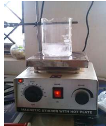
Figure 5. Magnetic stirring of MgO based nanofluid mixture
