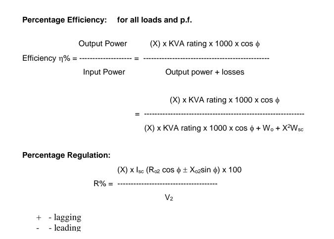
Where X is the load and it is 1 for full load,  $\frac{1}{2}$  for half load,  $\frac{3}{4}$  load,  $\frac{1}{4}$  load etc.. and the power factor is, upf, o.8 p.f lag and 0.8 p.f lead
