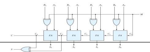
The mode input *M* controls the operation. When M = 0, the circuit is an adder, and when M = 1, the circuit becomes a subtractor.
